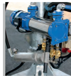
Насос, клапаны. Water distribution by solenoid valves and water filter installed on the A-60 industrial dust suppression fog cannon.
